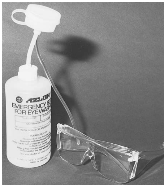
Plate 3.2 Left: 500ml emergency eye wash bottle. Squeezing the bottle gently sprays the eye. The waste liquid flows through a tube to the sink or collecting vessel. Instructions for use are printed in green on the bottle. Right: Protective eyeshields with closed in sides. The goggles are made from polycarbonate.
