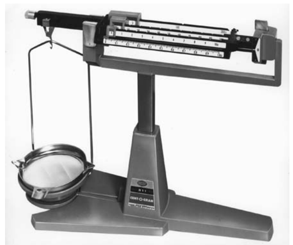
Plate 4.4 Ohaus 311 mechanical beam balance, readability of 0.01 g and capacity of 311 g, suitable for district hospital laboratories.
